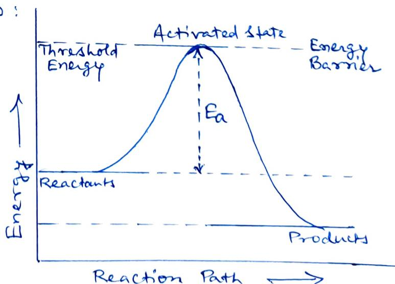
It is evident from the figure that there is a certain minimum energy (threshold energy) which the colliding molecules must acquire before they are capable of reacting. Most of the molecules,
