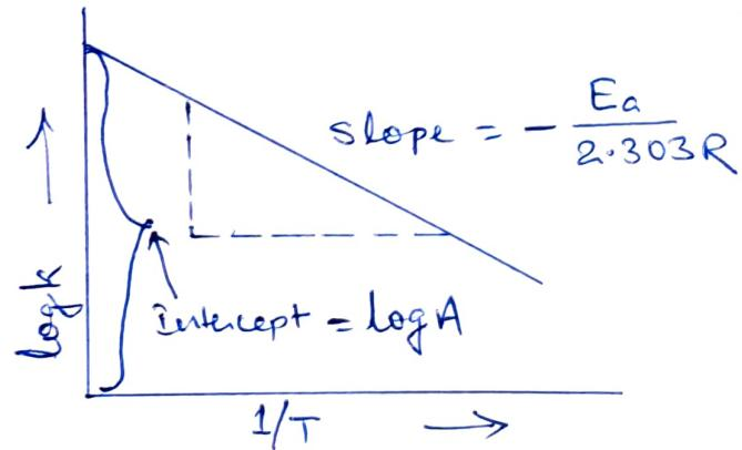
Calculation of  $E_a$  from the values of  $k$  at two Temperatures :-
